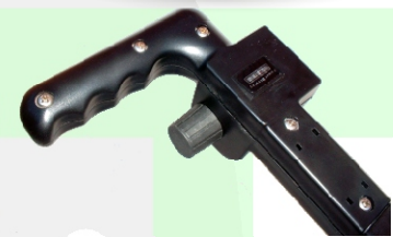
Variable control inc power meter
